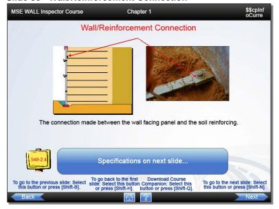
Slide 31 - Wall/Reinforcement Connection
