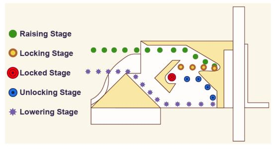
The disconnect assembly operates according to 5 basic stages:
